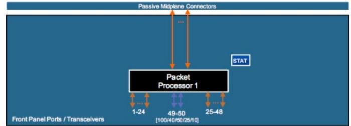
Figure 14: Arista DCS-7500R2AK-48YQ-LC (36 x 10G, 12 x 25G and 2 x100G)
