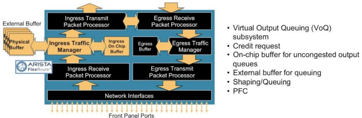
Figure 20: Packet Processor stage 3 (ingress): Ingress Traffic Manager
