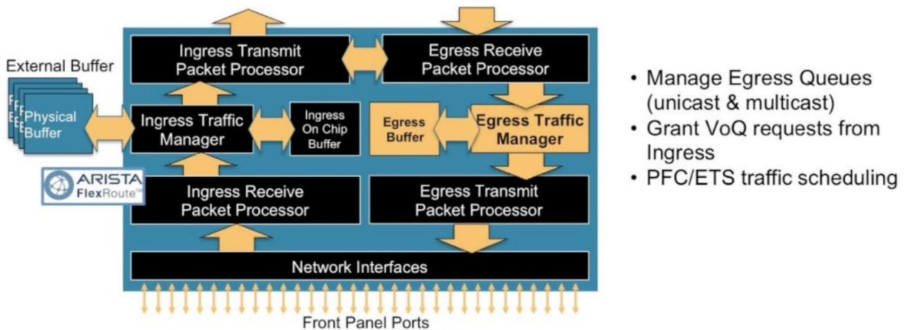
Figure 27: Packet Processor stage 7 (egress): Egress Traffic Manager
