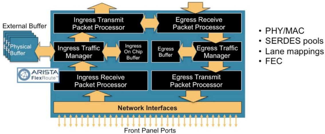
Figure 16: Packet Processor stage 1 (ingress): Network Interface
