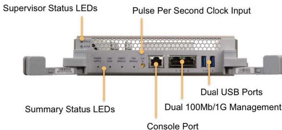
Figure 2: Arista 7500 Series Supervisor 2 Module.
