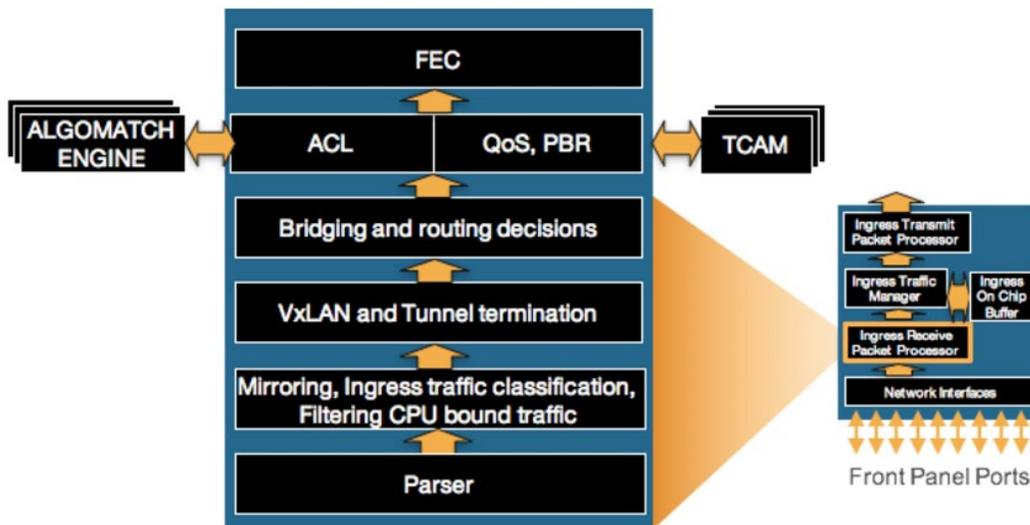
Figure 19: Ingress Receive Packet Processor with AlgoMatch
