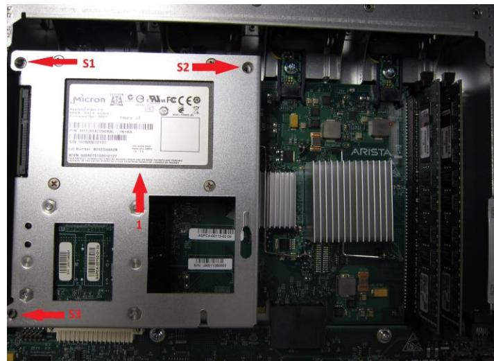
Figure 13-CPU Board SSD Memory Location
