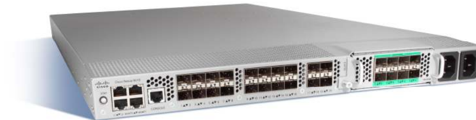
Figure 3. The Cisco Nexus 5000 Series Includes the Cisco Nexus 5010, Supporting 20 Fixed Ports of 10 Gigabit Ethernet (Ports 1 to 8 Can Run Gigabit Ethernet) and FCoE and One Expansion Module Slot
