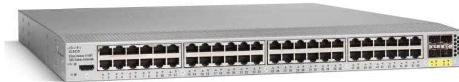
Figure 5. The Cisco Nexus 2148T Gigabit Ethernet Fabric Extender Supports 48 Fixed Ports of Gigabit Ethernet (1000BASE-T) Interfaces for Server Connectivity and Up to Four 10 Gigabit Ethernet Uplink Interfaces
