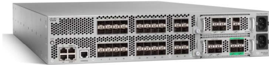
Figure 2. The Cisco Nexus 5000 Series Includes the Cisco Nexus 5020, Supporting 40 Fixed Ports of 10 Gigabit Ethernet (Ports 1 to 16 Can Run Gigabit Ethernet) and FCoE and Two Expansion Module Slots
