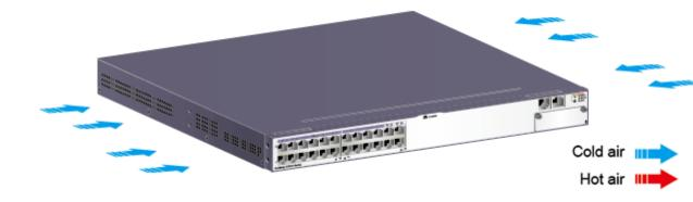
**NOTE** This figure only shows the airflow direction and does not depict the actual device.
