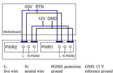
Figure 6-45 Power supply by dual AC PoE power modules
