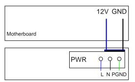
Figure 6-97 Power supply mode of a built-in AC power module
