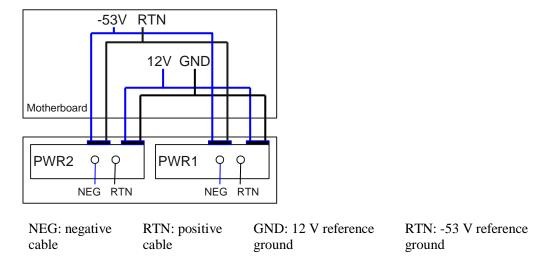
Figure 6-49 Power supply connections of dual DC PoE power modules
