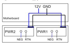
Figure 6-71 Power supply connections of dual DC power modules
