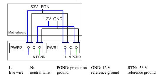
Figure 3-201 shows the power supply connections of dual DC PoE power modules. After DC power is transmitted to the PWR module, the PWR module provides 12 V and -53 V output voltages, and the motherboard provides 12 V voltage for the entire device and -53 V voltage for the PDs.
