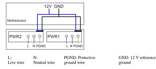
Figure 6-32 Power supply connections of dual non-PoE AC power modules
