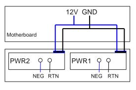
NEG: negative cable RTN: positive cable GND:
