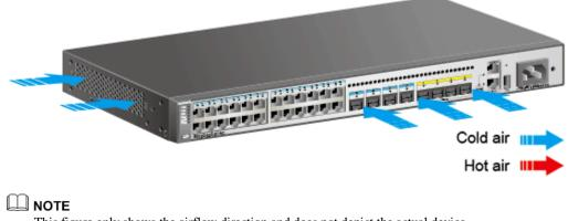
This figure only shows the airflow direction and does not depict the actual device.
