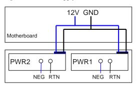
Figure 6-51 Power supply connections of dual DC power modules
