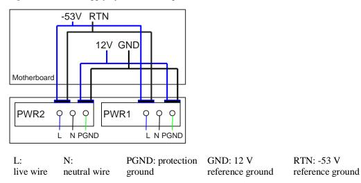
Figure 6-63 Power supply by dual AC PoE power modules
