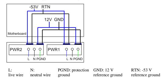
Figure 6-69 Power supply by dual AC PoE power modules
