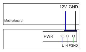
L: live wire N: neutral wire PGND: protection ground GND: 12 V reference ground
