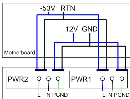
L: live wire      N: neutral wire      PGND: protection ground      GND: 12 V reference ground      RTN: -53 V reference ground
