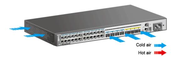
**NOTE** This figure only shows the airflow direction and does not depict the actual device.
