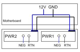
NEG: negative cable RTN: positive cable GND: 12 V reference ground
