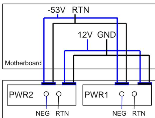
NEG: negative cable      RTN: positive cable      GND: 12 V reference ground      RTN: -53 V reference ground
