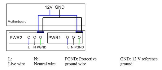
Figure 6-55 Power supply connections of dual non-PoE AC power modules
