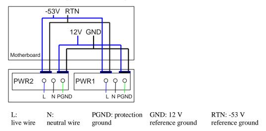
Figure 6-66 Power supply by dual AC PoE power modules
