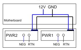
Figure 6-24 Power supply connections of dual DC power modules
