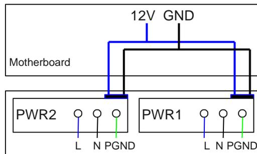
L: Live wire      N: Neutral wire      PGND: Protective ground wire      GND: 12 V reference ground
