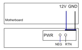
NEG: negative cable RTN: positive cable GND: 12 V r
