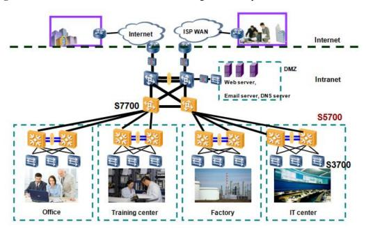
Figure 5-1 Position of the S5700-EI/S5720-EI on a large-scale enterprise network
