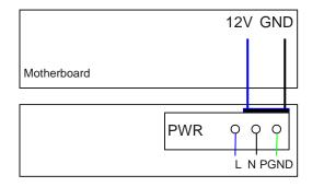
L: live wire N: neutral wire PGND: protection ground GND: 12 V reference ground
