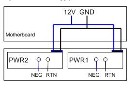
NEG: negative cable RTN: positive cable GND: 12 V reference ground
