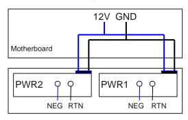
RTN: positive cable NEG: negative cable GND: 12 V reference ground
