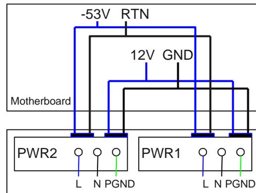
L: live wire      N: neutral wire      PGND: protection ground      GND: 12 V reference ground      RTN: -53 V reference ground
