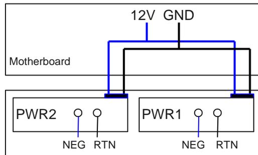
NEG: negative cable      RTN: positive cable      GND: 12 V reference ground
