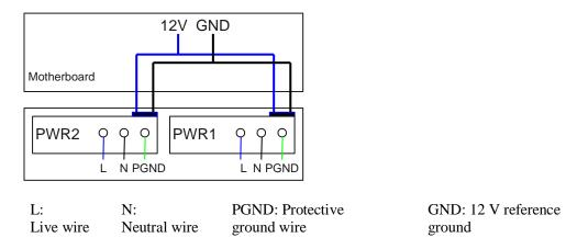
Figure 6-13 Power supply connections of dual non-PoE AC power modules
