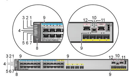
Figure 6-21 Indicators on the S5710-28C-PWR-EI-AC
