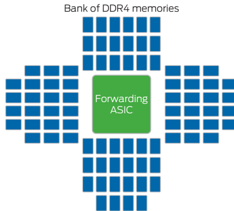
Figure 9: 1 Tbps forwarding ASIC with 4 GB external memory using DDR4 technology
