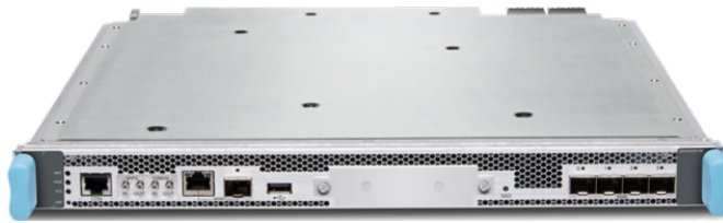
Figure 6: Routing Engine on the modular QFX10000 platform
