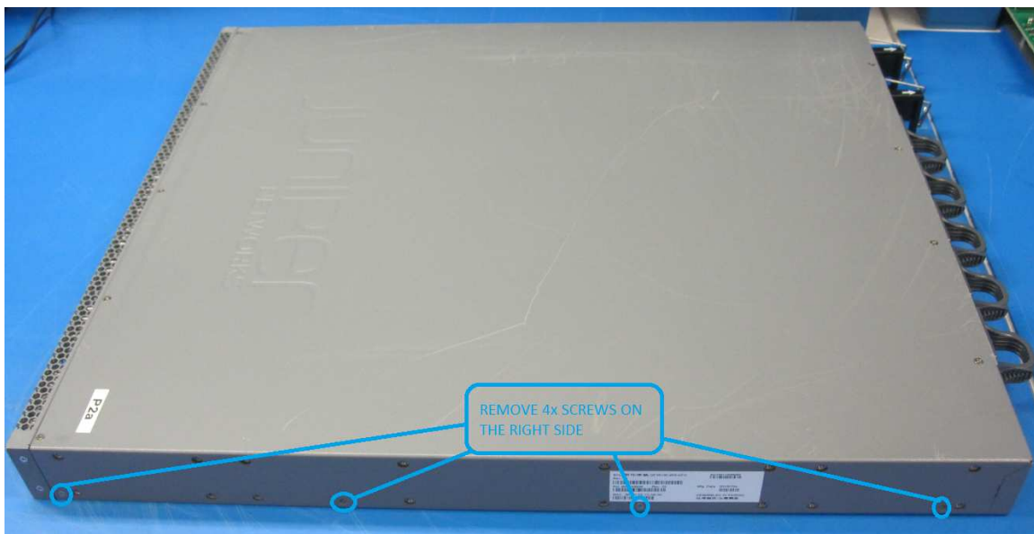
Figure 3-3: Right side screws
