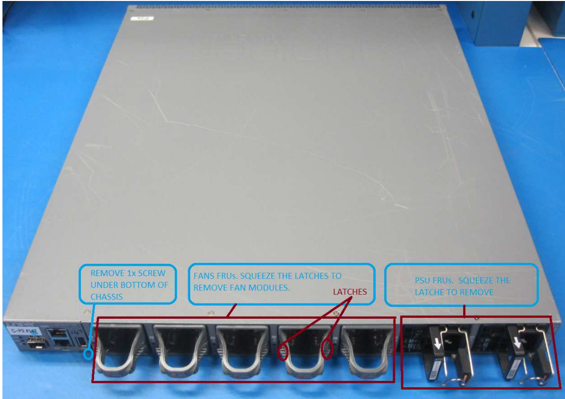
Figure 3-4: Rear screw + FAN FRUs + PSU FRUs
