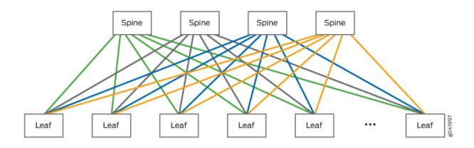
A VCF is based on either QFX5100 or QFX5110 switches as the spine devices, as follows:
