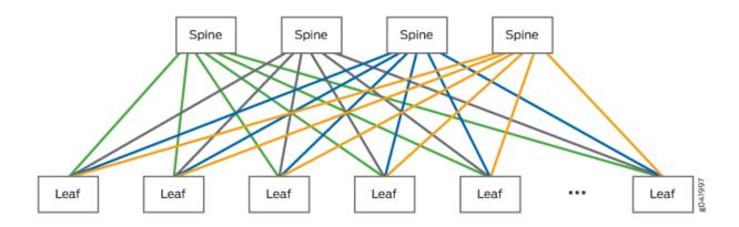
**NOTE:** A VCF topology should include at least four members—two spine devices and at least two leaf devices. For topologies with three or fewer members, use a Virtual Chassis configuration instead.
